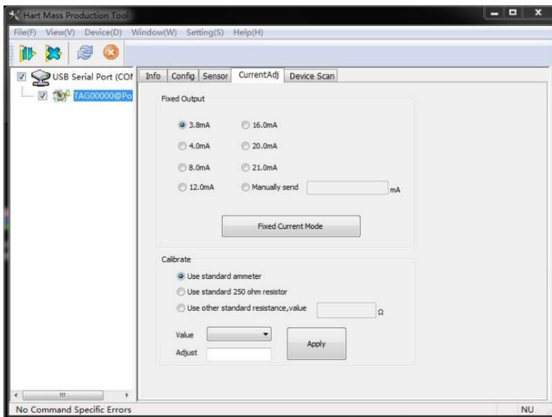
Figure 5.1 Current calibration
