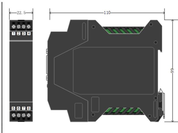
Figure 2.1 Dimension of Temperature Transmitter (Unit: mm)
