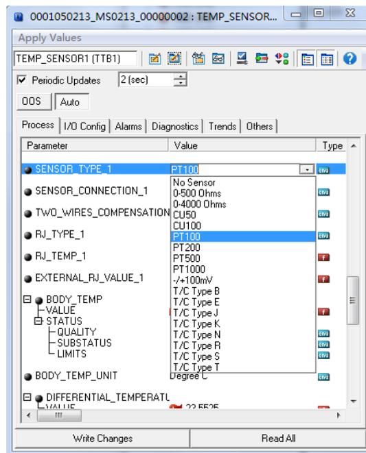
Figure 3.3 Configuration of sensor types
