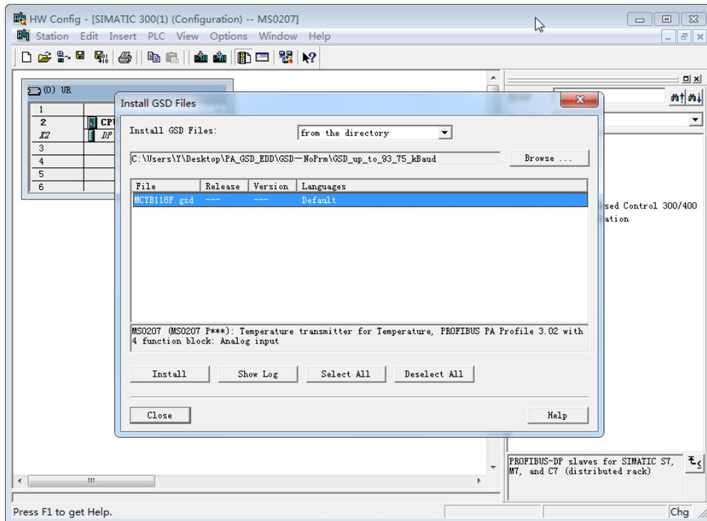
Figure 4.5 Install the GSD file
