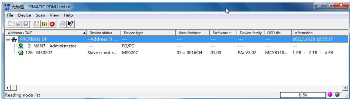
Figure 4.10 Scan DP Bus lists the PA devices
