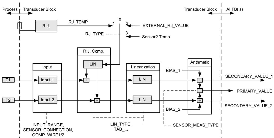
Figure 4.1 Conversion block structure
