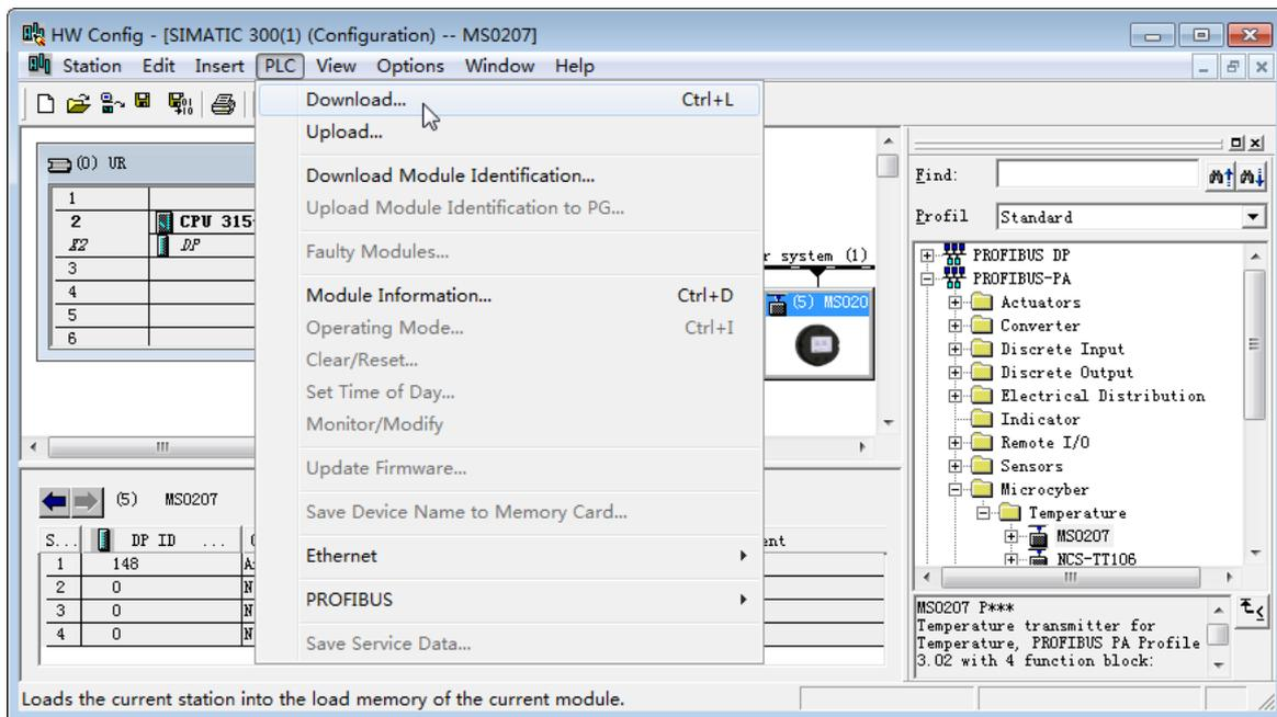
Figure 4.7 Download the configuration information to the PLC
