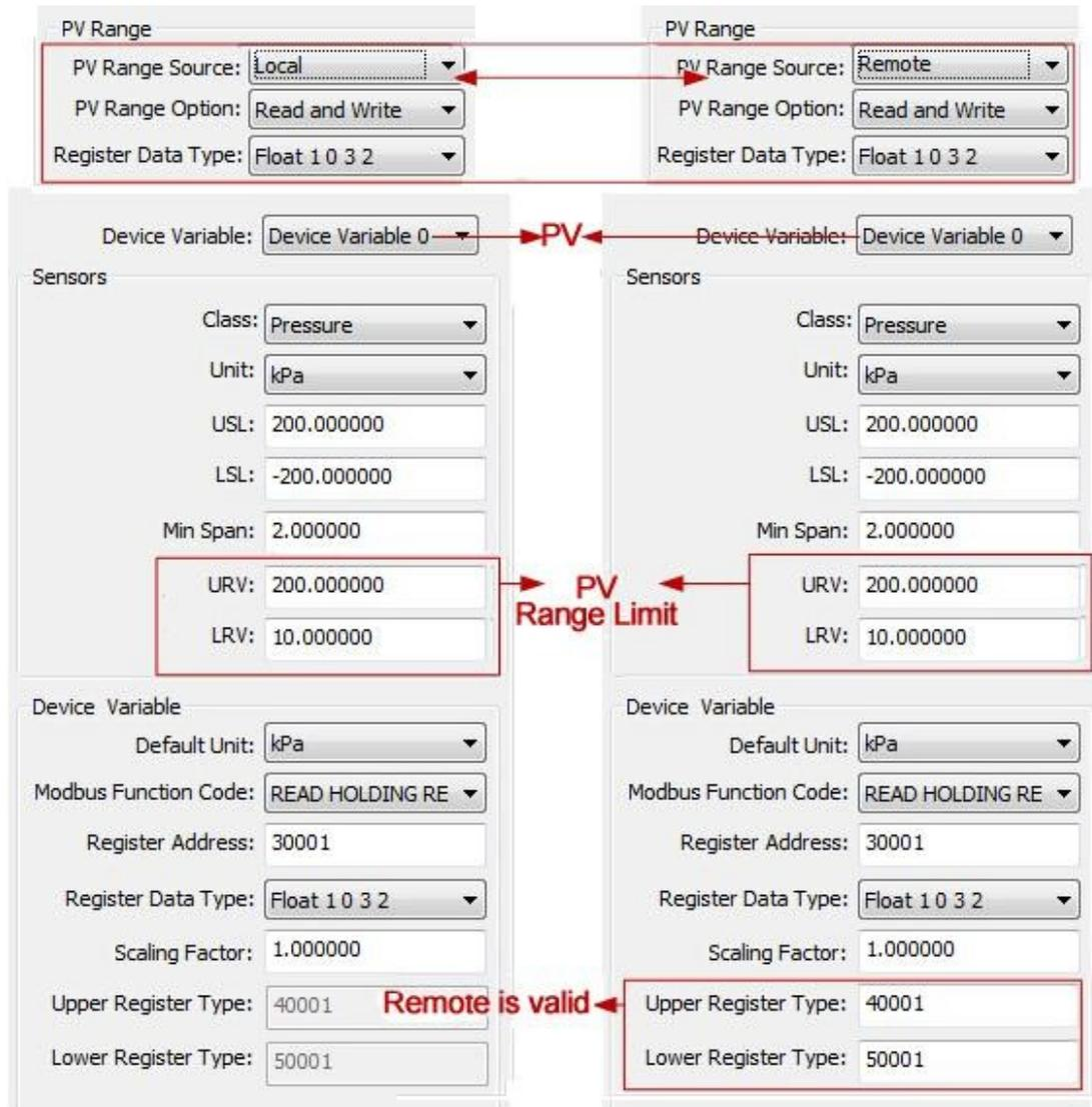
Figure 3.5 Example of PV range operation
