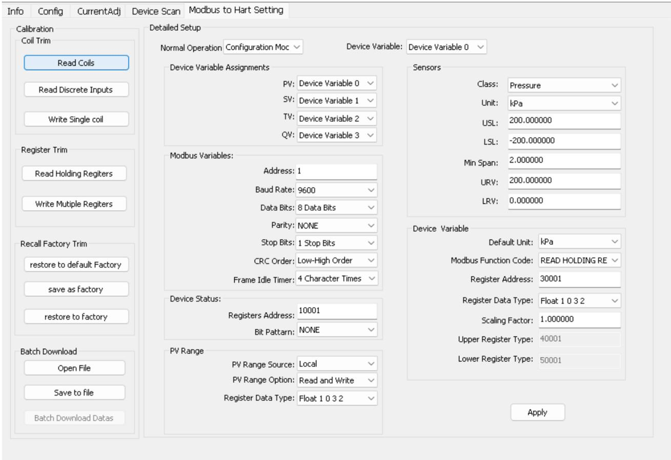
Figure 2.4 Gateway Configuration tab
