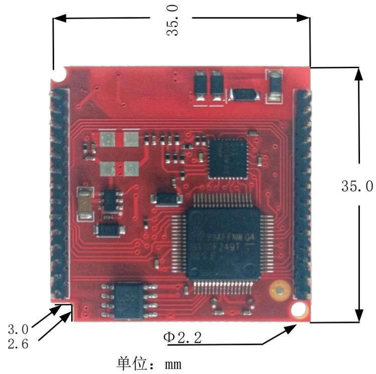
Figure 1.4 Mechanical dimensions of the front of the HART module (unit: mm)
