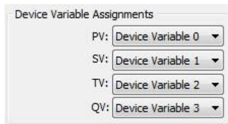
Figure 2.8 Device variable to dynamic variable assignment
