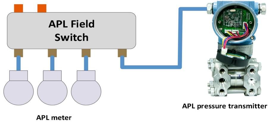
Figure 22 Application of MC0312 module in pressure transmitter
