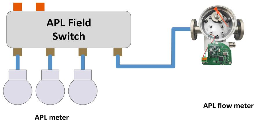
Figure 23 Application of MC0312 module on flow meter
