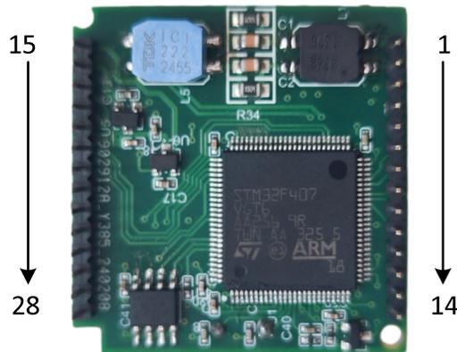
Figure 4 MC0312 built-in core module interface definition
