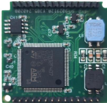
Figure 1 MC0312 Ethernet-AP Built-in Core Module
