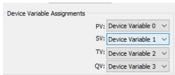
Figure 14 Assignment of device variables to dynamic variables
